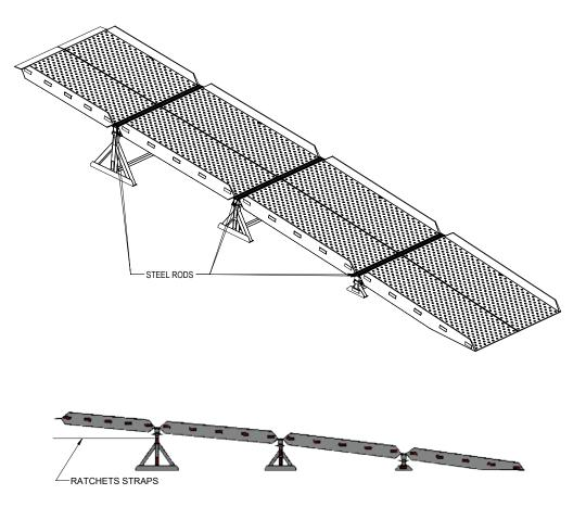
Step 6. Install the two ratchet safety straps, attaching them from the upper stand to the trailer.
