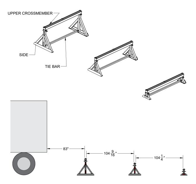
**Step 2.** Install one of the upper ramps making sure the tallest stand is in position to the trailer/dock. Reposition the stands as necessary. Install the other upper ramp.
