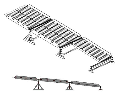
**Step 5.** Install the lower ramps. With all the ramps in place, install the steel rods to secure the ramps to the stands. Make sure each rod is secured with an R-clip.
