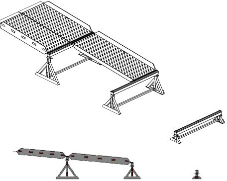
**Step 4.** With both upper ramps installed, and the upper middle ramps installed, repeat with the lower middle ramps. Check the position of the lowest stand. Adjust as needed. Install the last middle ramp. (All four middle ramps are the same.)
