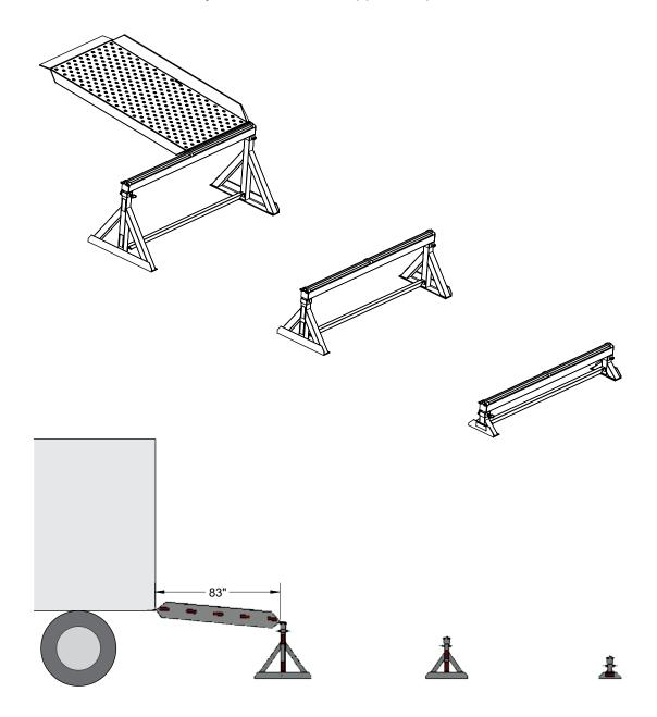
**Step 3.** With both upper ramps installed, install one of the upper middle ramps. Check the position of the middle stand, and adjust as needed. Install other upper middle ramp. (All four middle ramps are the same.)
